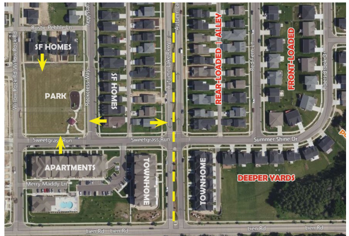
This neighborhood incorporates varied housing types, using building orientation to mitigate compatibility issues.
