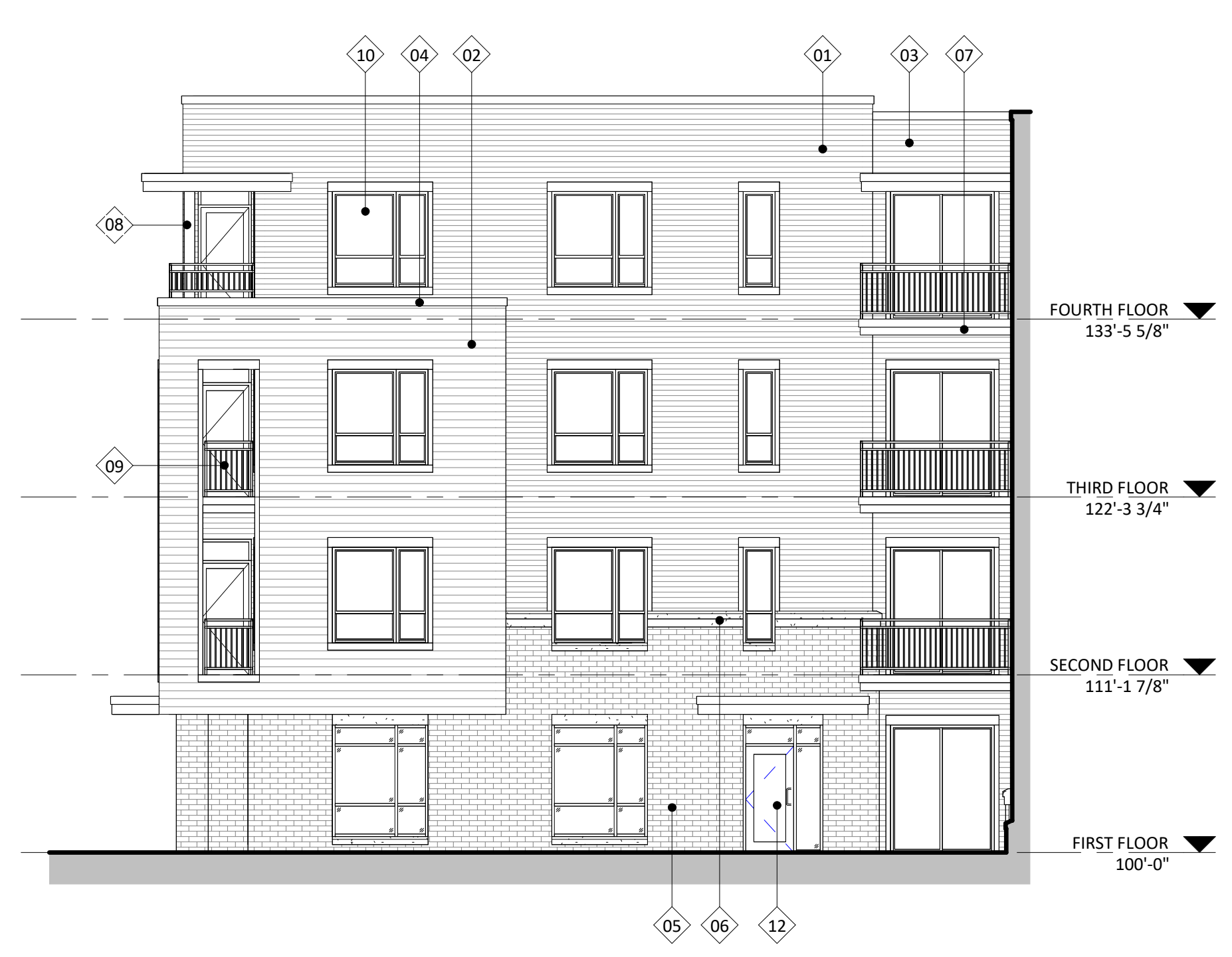
2 ELEVATION - NORTHEAST COURTYARD 1/8" = 1'-0"
