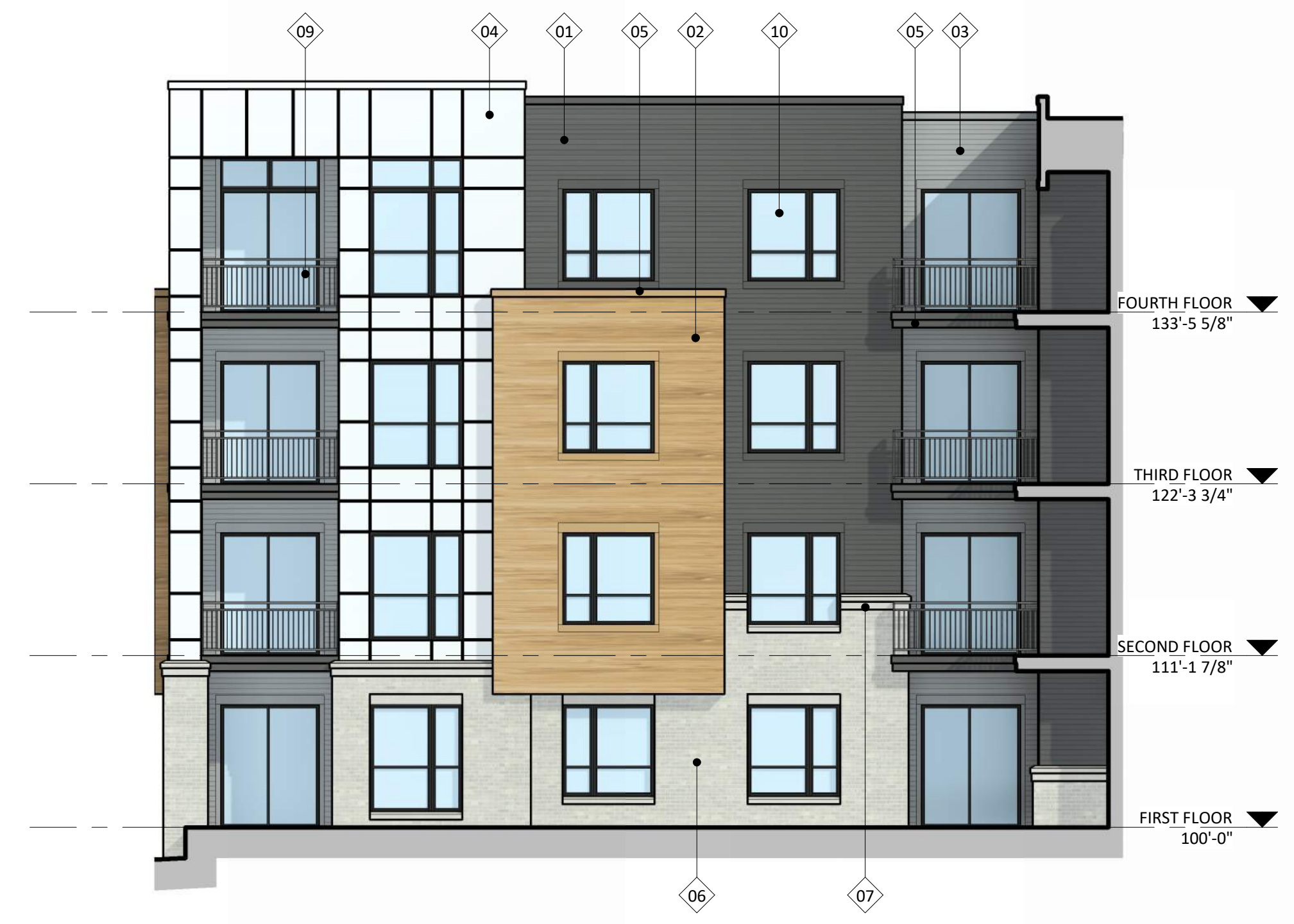
2 COLORED ELEVATION - NORTHEAST COURTYARD AC204.2 1/8" = 1'-0"
