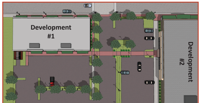
This illustration shows two developments on adjoining lots sharing parking and an access drive. A sidewalk connects the two developments through the parking area.
