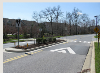
Raised Median / Crossing Refuge, Plus Speed Table
