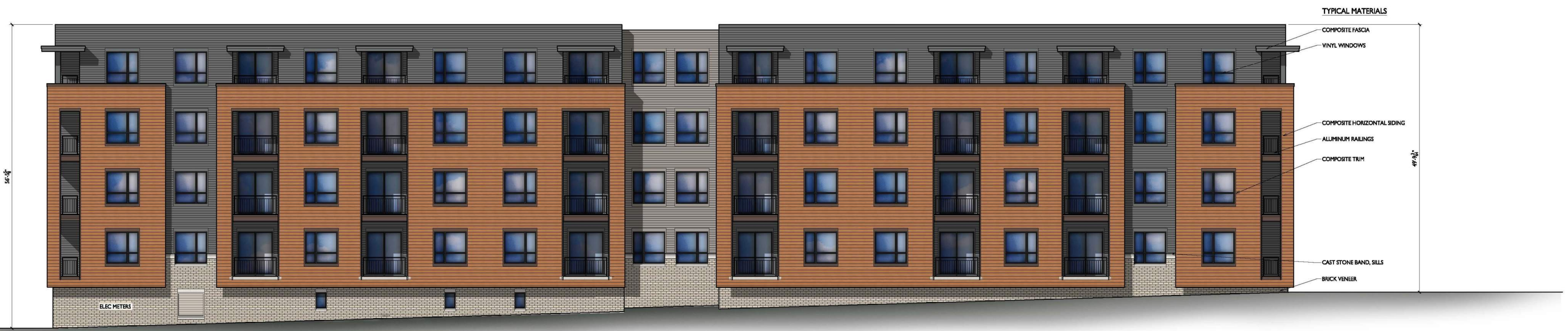
BUILDING 1 SOUTHEAST ELEVATION ALONG NESBITT 2 AC201.1 3/32" = 1'-0"
