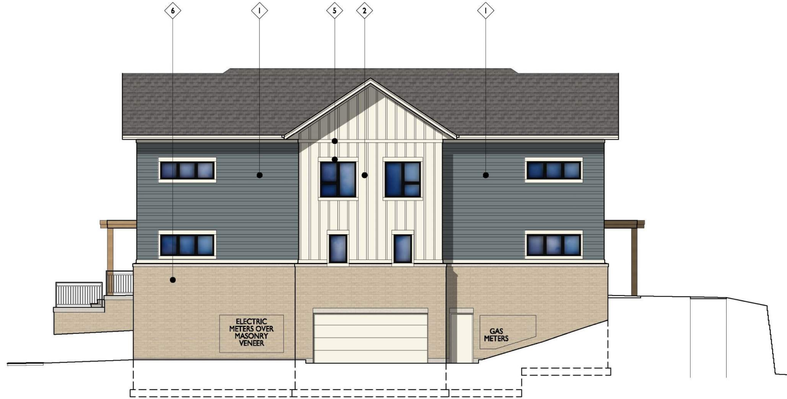
BUILDING A EAST ELEVATION A203.A 1/8"=1'-0"
