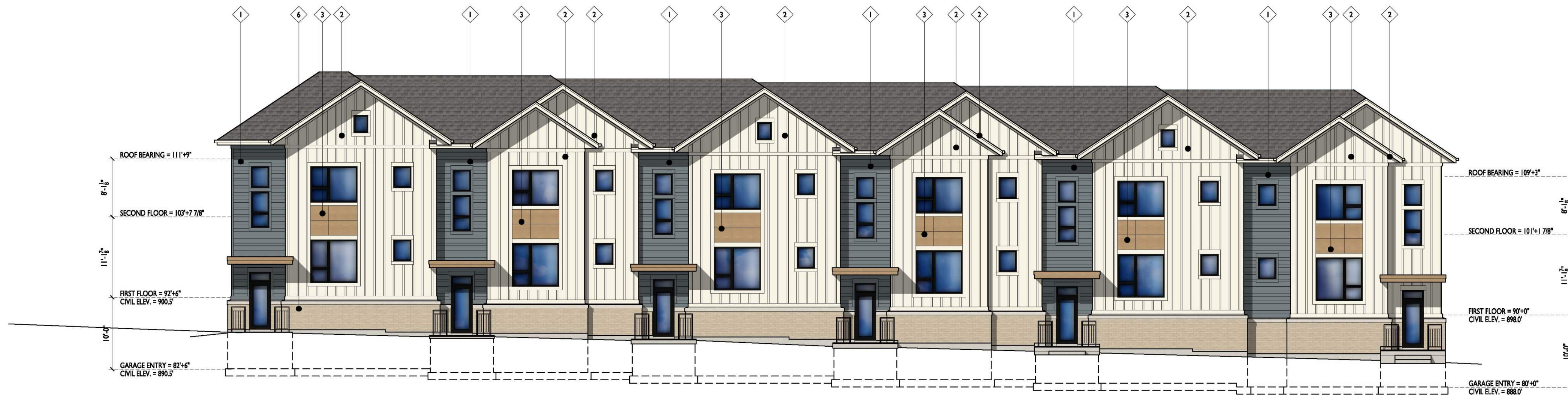
BUILDING B SOUTH ELEVATION 1 A203.B 1/8"=1'-0"
