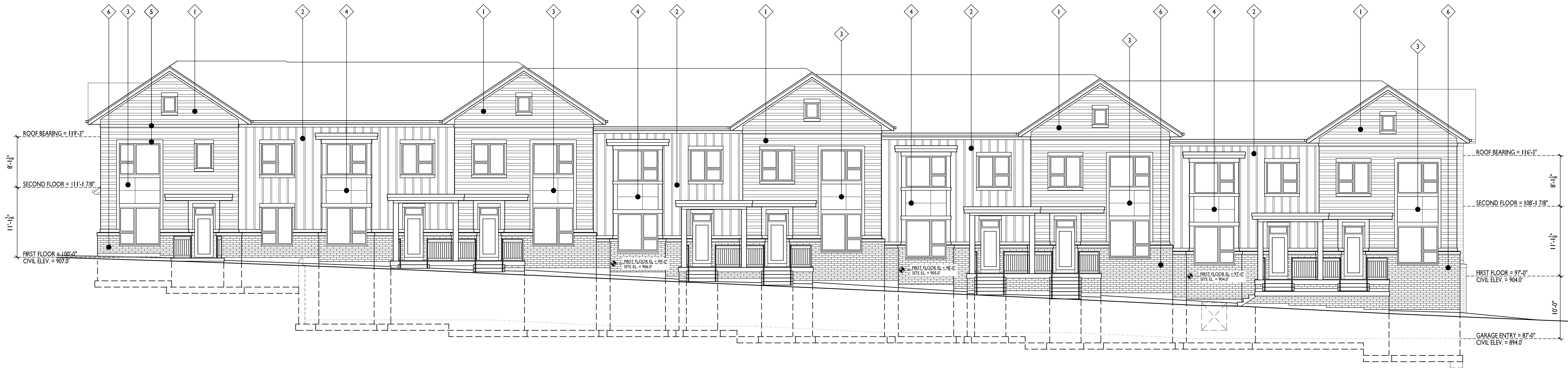
BUILDING A SOUTH ELEVATION 1 A201.A 1/8"=1'-0"
