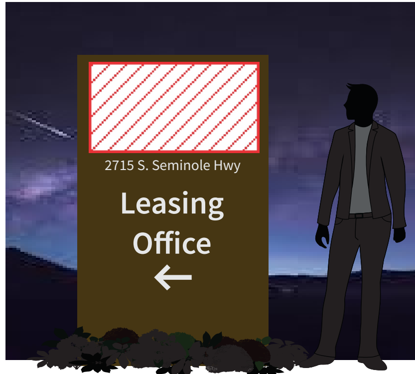
Fabricated Aluminum Cabinet, w/ Posts Mounted Below Grade Colors TBD 7.77 Sq Ft Per Side
