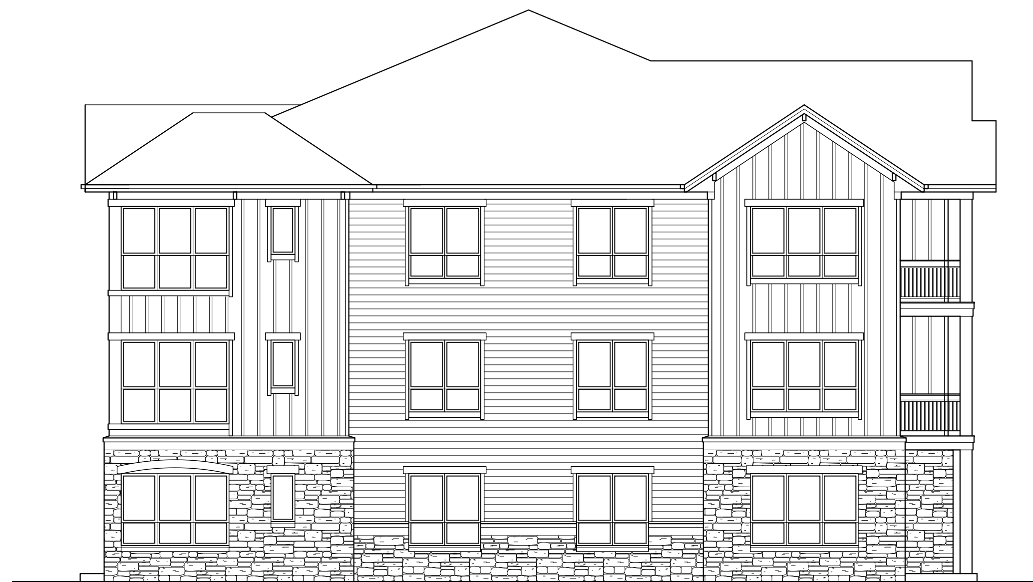
1 EAST ELEVATION (BUILDING 1) A-2.2 1/8" = 1'-0"
