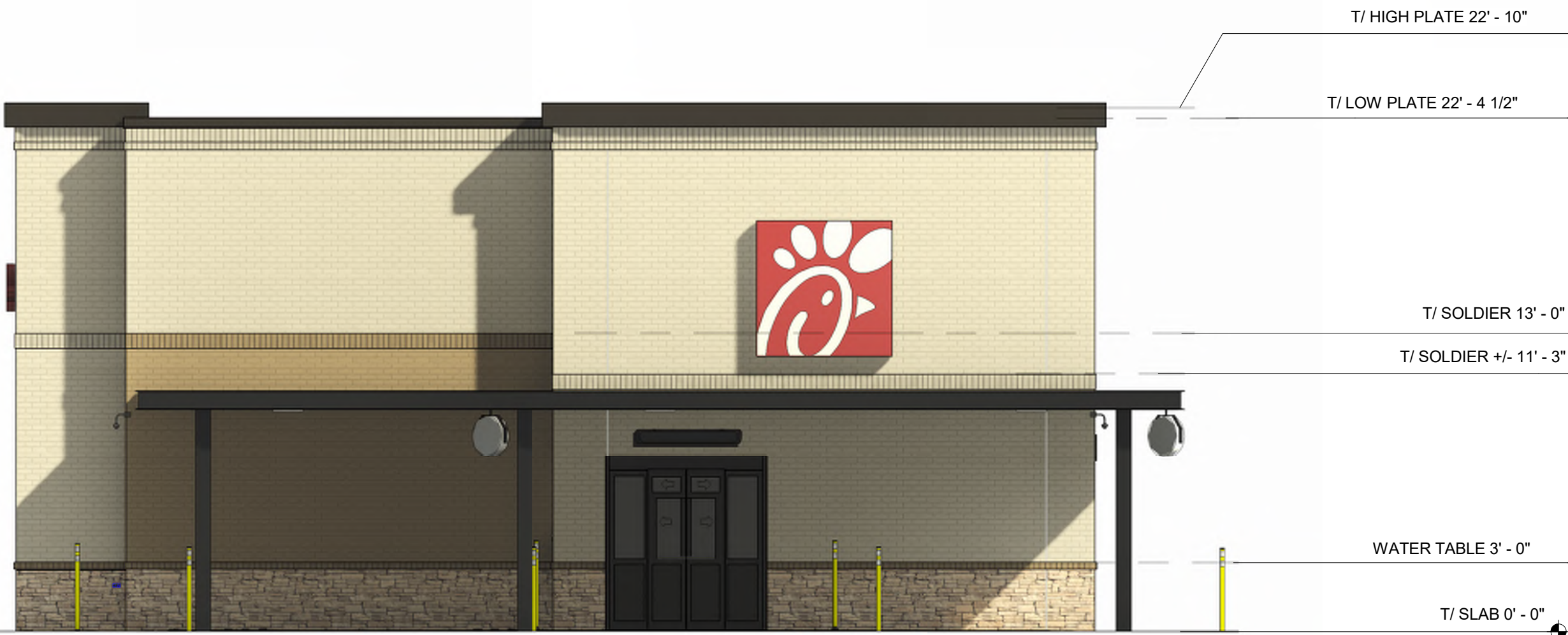
EAST EXTERIOR ELEVATION 3/16" = 1'-0"
