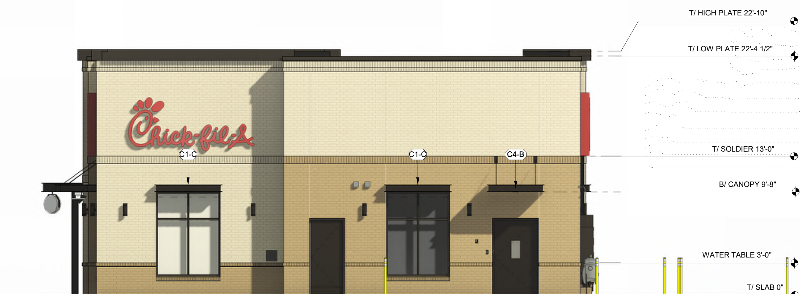
WEST EXTERIOR ELEVATION
