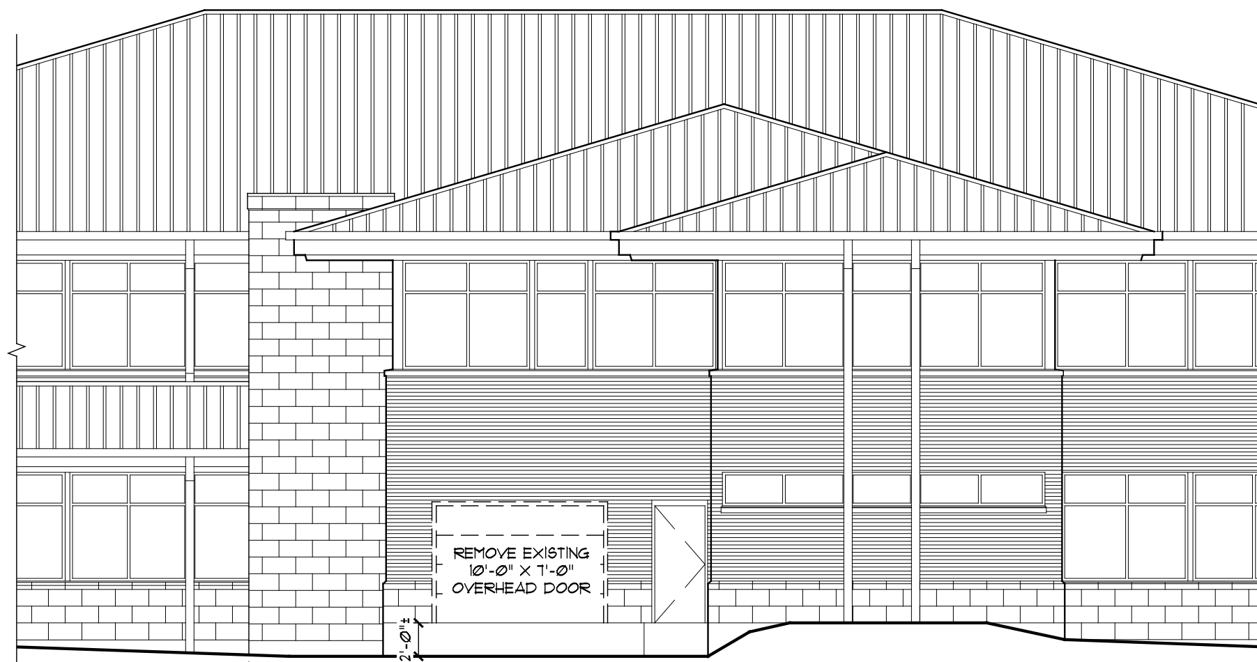
3 EXISTING NORTHWEST EXTERIOR ELEVATION C-1.1 SCALE: 1/8" = 1'-0"
