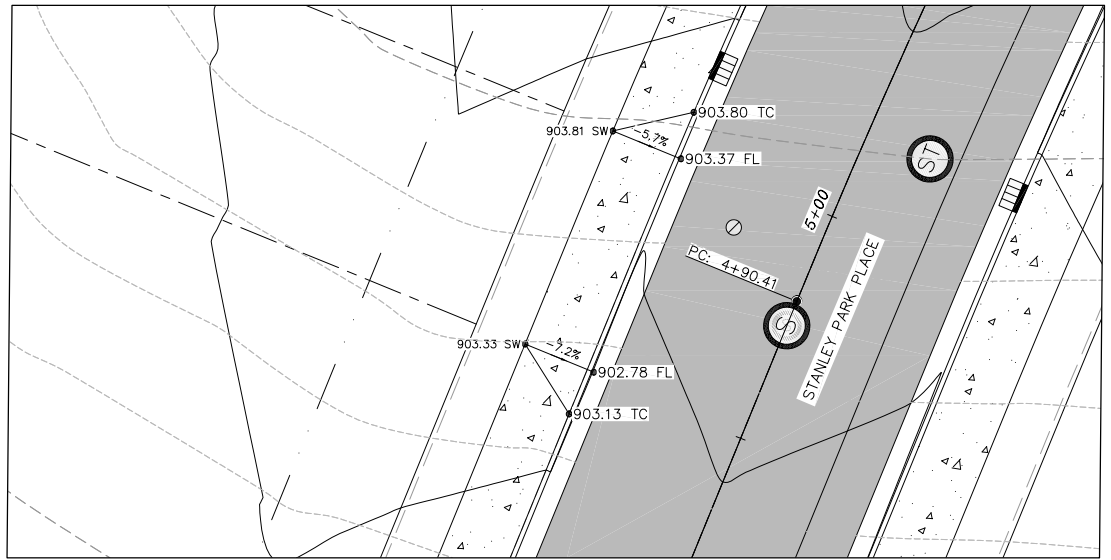
2 DRIVEWAY GRADING DETAIL 1" = 10'
