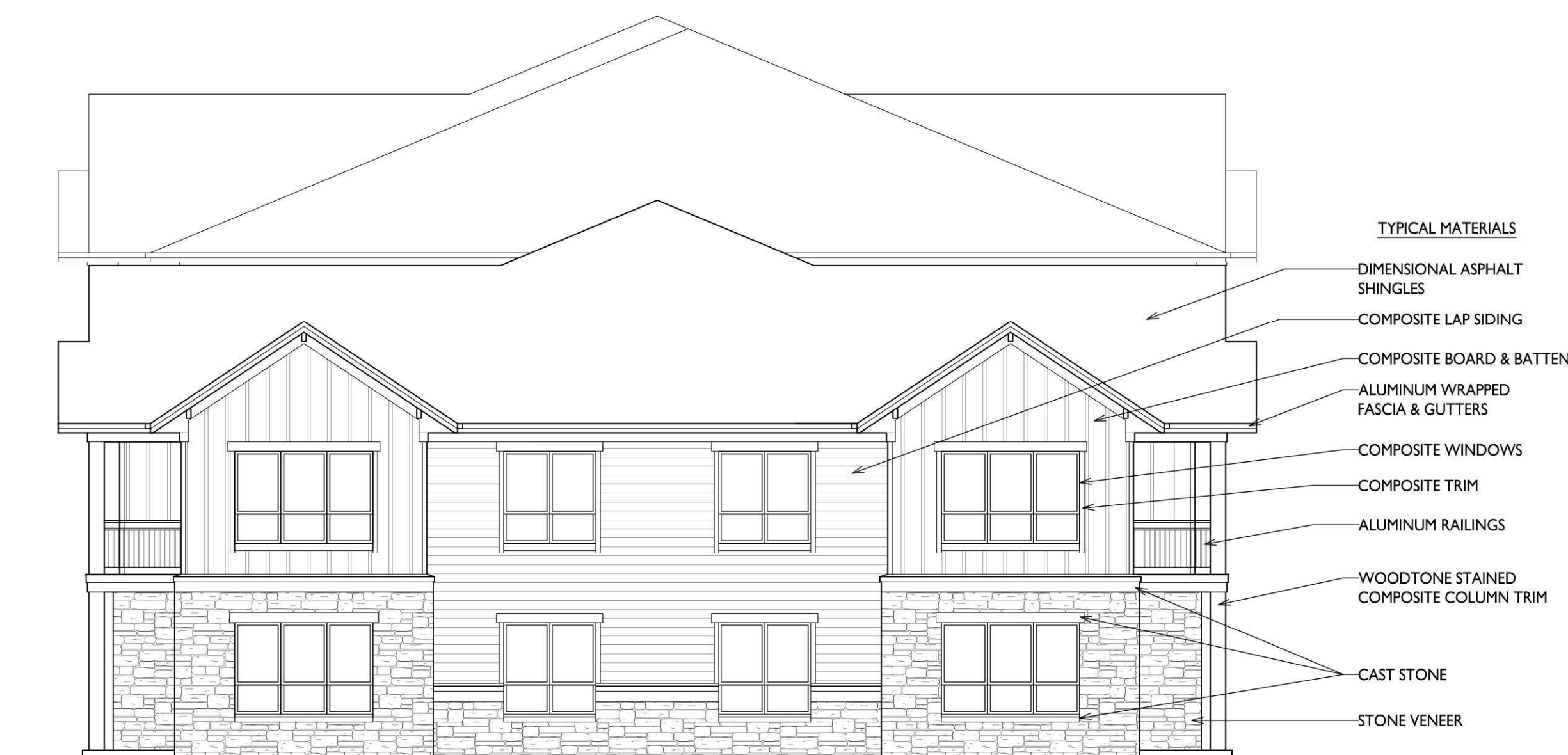
2 EAST ELEVATION - BUILDING 4 A-2.5 1/8" = 1'-0"
