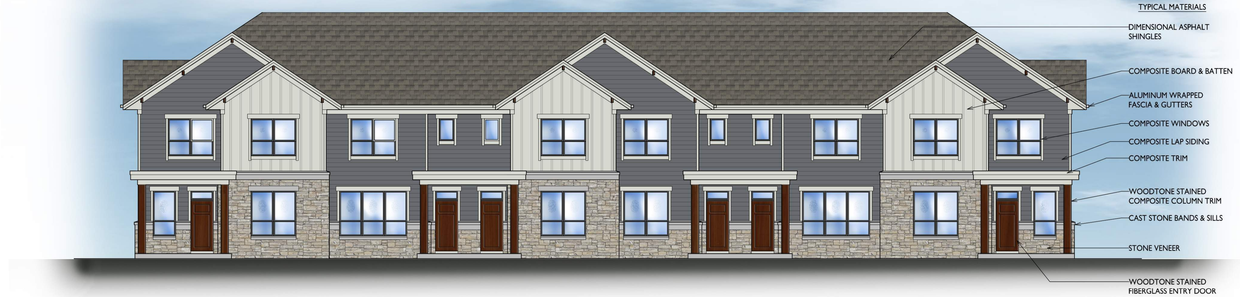
1 SOUTH ELEVATION - BUILDING 5-8 A-2.7 1/8" = 1'-0"
