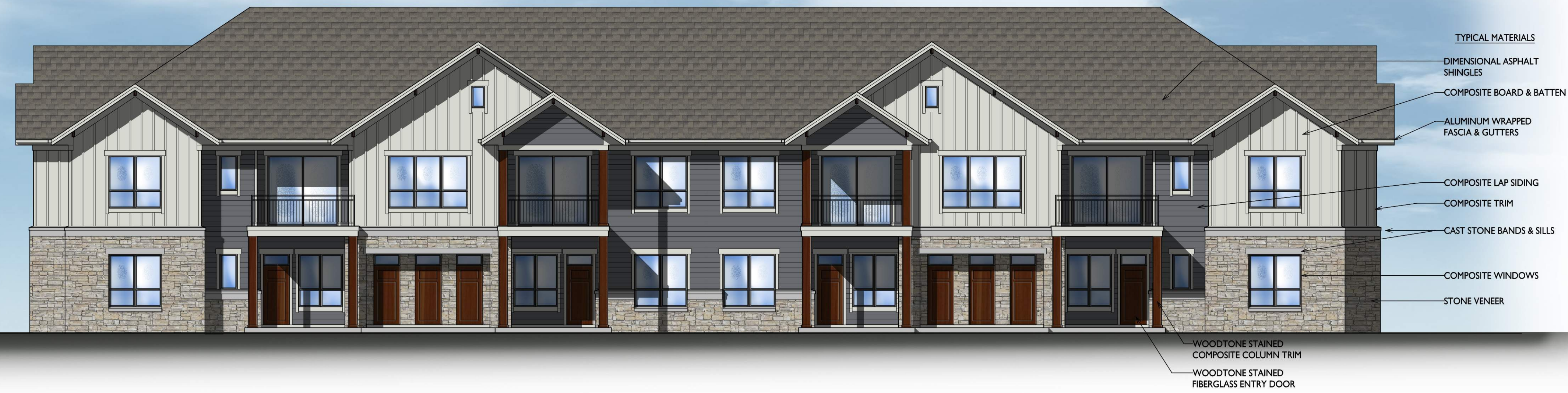
1 SOUTH ELEVATION - BUILDING 9-10 A-2.9 1/8" = 1'-0"
