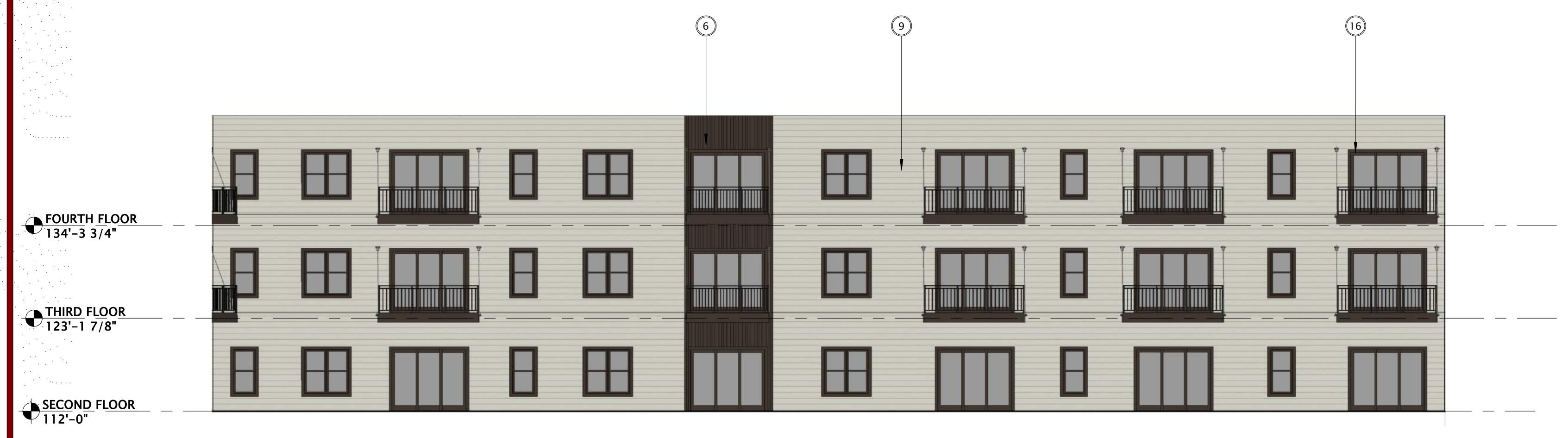
11 COURTYARD NORTH ELEVATION 3/32" = 1'-0"
