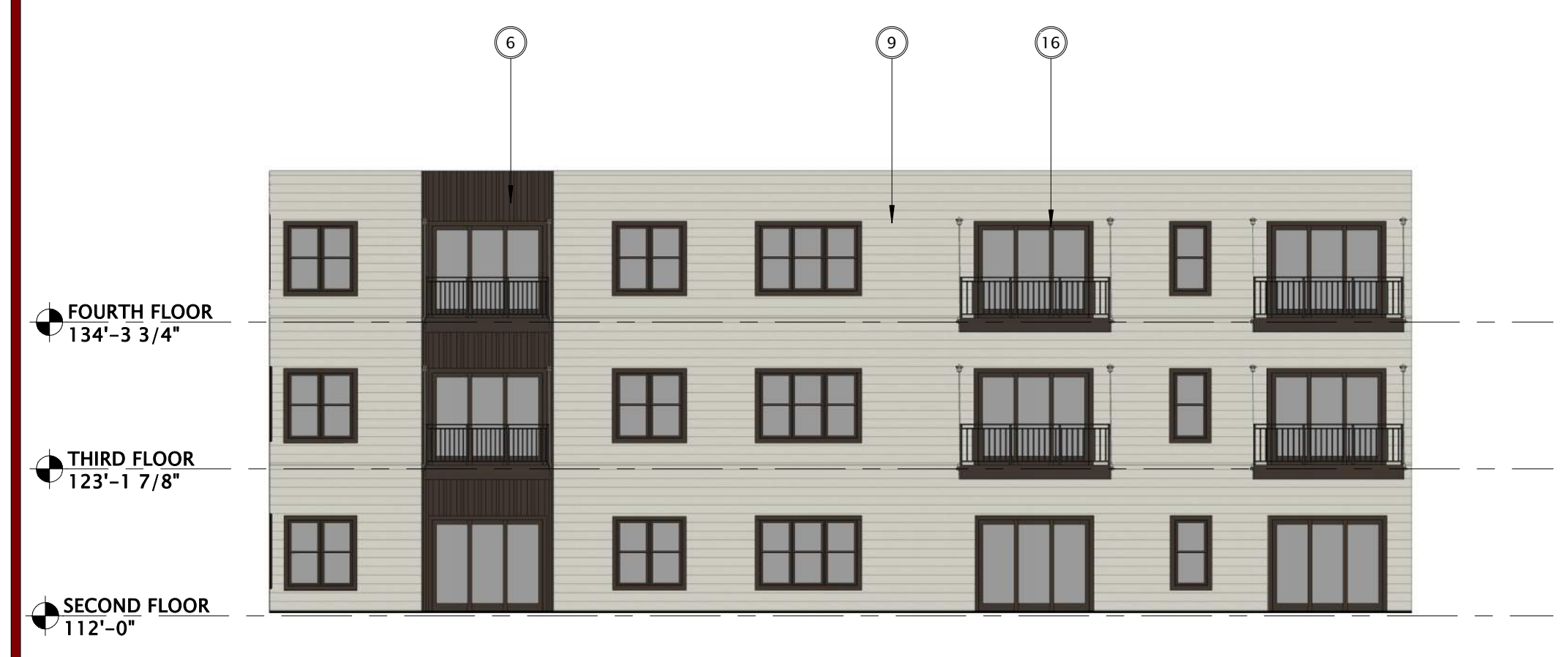
16 COURTYARD WEST ELEVATION 3/32" = 1'-0"
