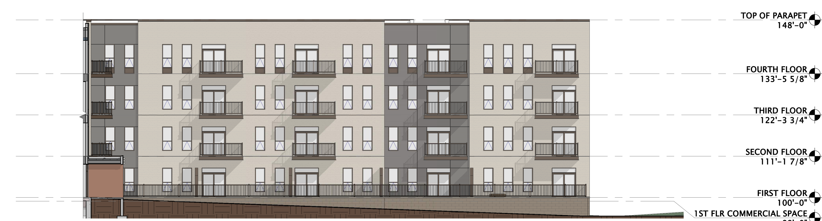
4 OVERALL NORTHEAST ELEVATION (PARKING LOT) 1/16" = 1'-0"
