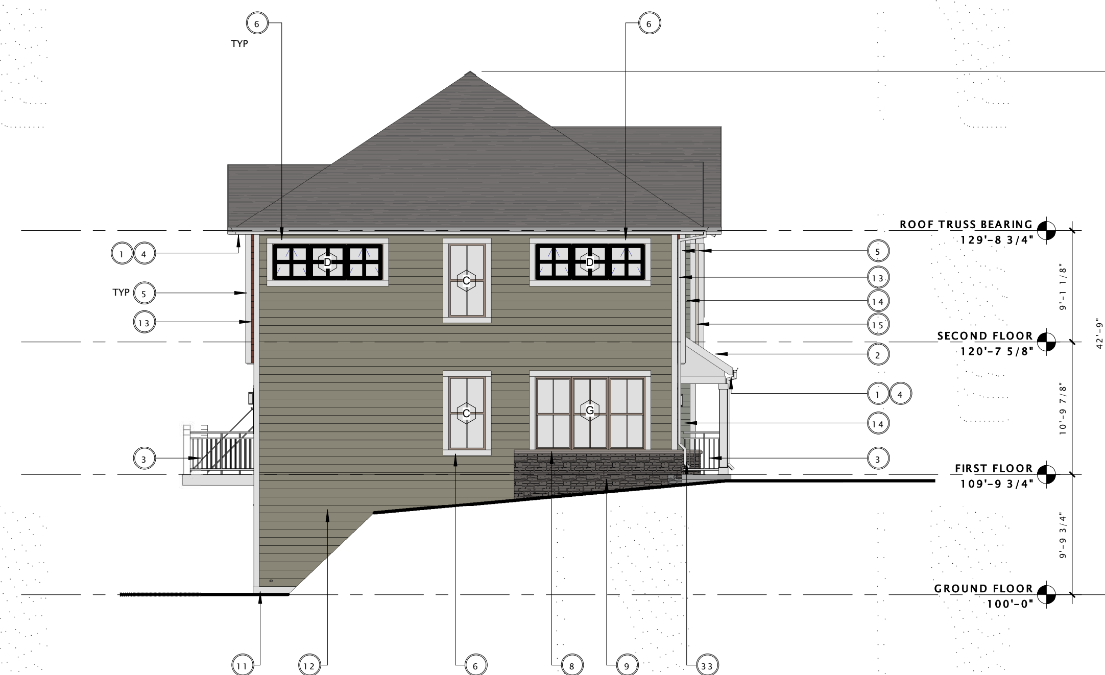
16 BUILDING T1 - WEST ELEVATION 1/8" = 1'-0"
