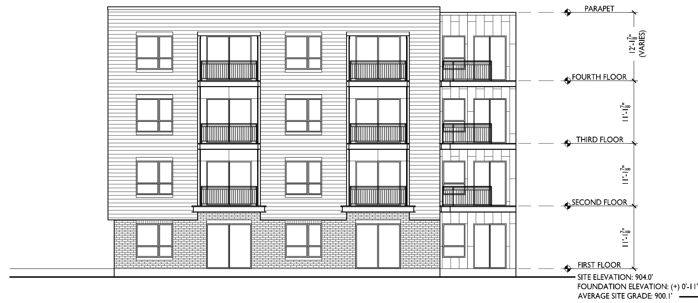
3 EAST COURTYARD ELEVATION A-2.2 3/32"=1'-0"
